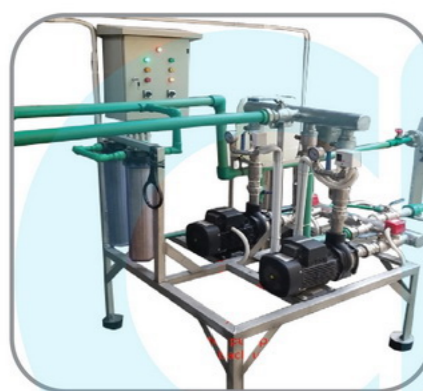
Water Pump dan Redundant control panel
